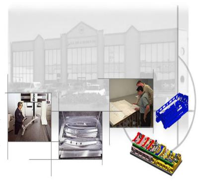
At G.S. Die & Design, dies begin with quality engineering using the latest in technology, and skilled personnel. The first step is analysis of the part geometry using Dynaform's Blank Size Engineering module to determine blank size & shape, as well as any problem areas that might be of concern while forming. By applying their advanced F.E.A. technology at the die concept stage, G.S. Die is able to identify and address potential manufacturing concerns at the early stages of tool development.
