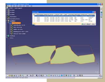
CATNEST will determine the material utilization for standard cutoff die shapes
