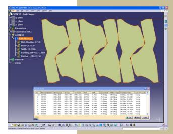
Nest in 1-up, 2-up, or mirrored layouts to optimize material utilization
